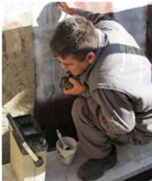
a) Process of ultrasonic testing b) Location of the 10 mm deep surface crack in the area of the butt - welded joint Figure 7. Determination of depths of surface cracks in the area of the butt-welded joint
