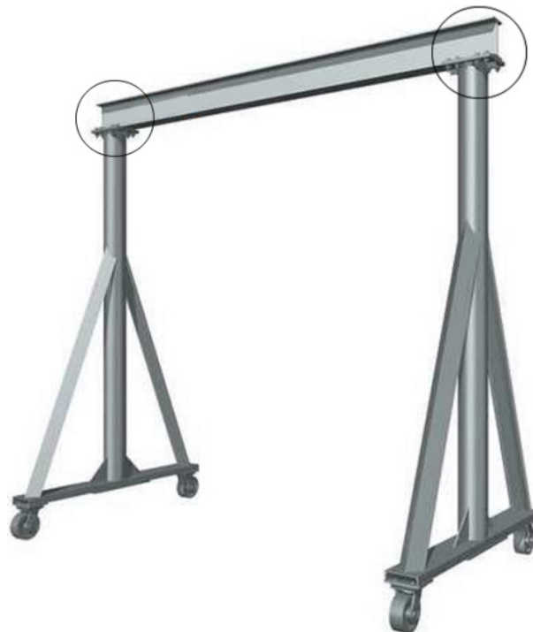
Figure 2. Steel frame of the gantry crane.
