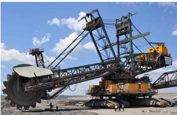
Fig. 1. BWE SchRs 1600 (Serbian mining basin Kolubara): mass (with the mobile conveyor) 3345 t, declared theoretical capacity 6600 m 3 /h.
