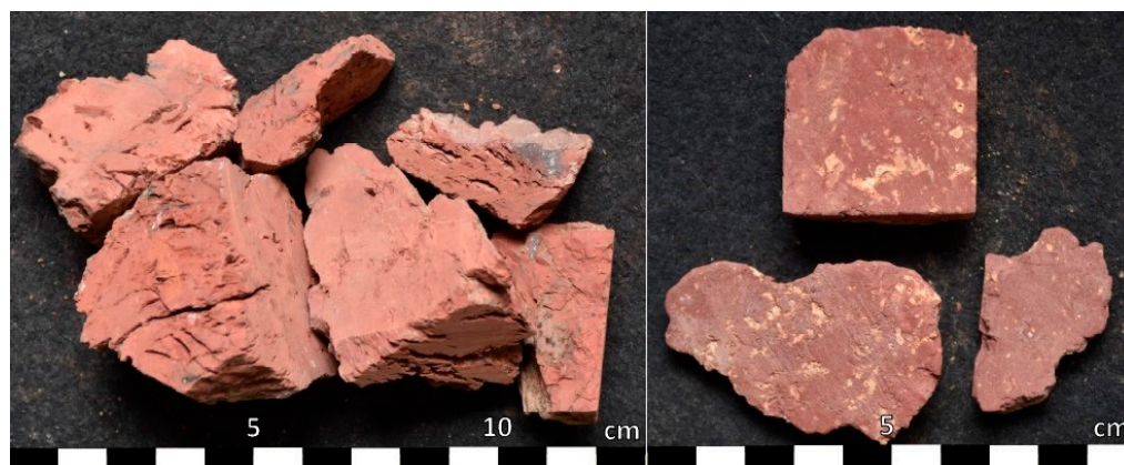
Figure 8. Two samples of natural brick from the bed, cut for the testing in laboratory. Sample 1 (left), sample 2 (right). Photo-documentation of the MoDeCo2000 project.
