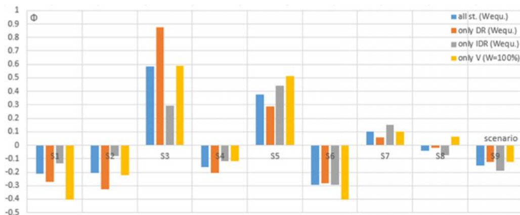
Figure 12: Final solutions obtained by optimization only across all maximum global drifts DR_{max} (weight assigned to the criteria are equivalent for all floors), only across all inter-storey drifts IDR for the level of maximum global drift DR_{max} (weights assigned to the criteria are equivalent for all floors), and only across the total shear force in the base of the object V for the level of global drift DR_{max} (weights assigned to the criteria are equivalent for all floors)
