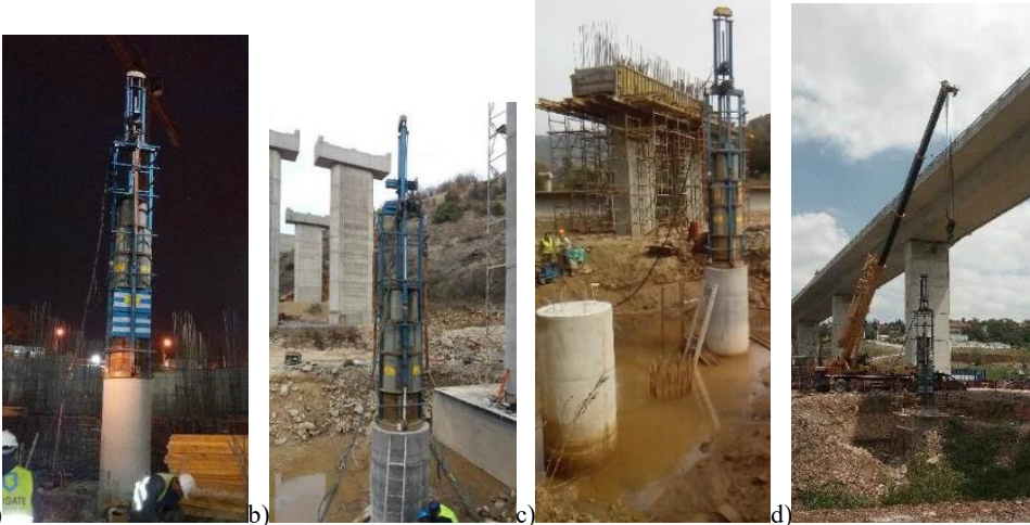
Figure 6. DLT – equipment set for the tests in Serbia: a) office-commercial building-tower Ušće 2, b) Gradsko-Prilep express road bridges in Macedonia, c) bridges on corridors X and XI, d) viaducts on the E 70/E 75 highway
