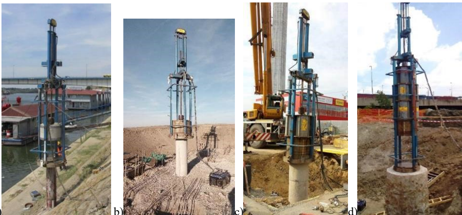
Figure 5. DLT – equipment set for the tests in Serbia: a) Sava Promenade, b) Malibunar wind farm, c) Aviv Park in Belgrade, d) access road for the Ada bridge
