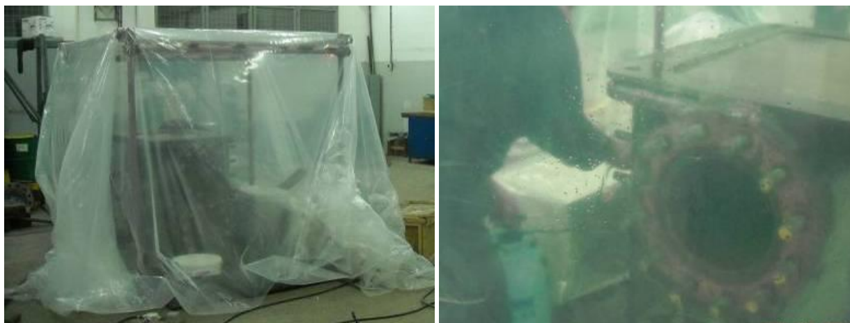
Figure 2. Workshop conditions degreasing biodegradation of housing of oil distribution
