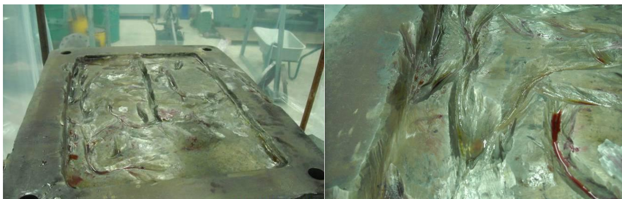
Figure 3. The treated surface and the traces of degraded oil which left the porous structure of the metal
