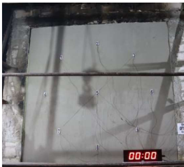
Fig. 2. Fire resistance test of walls (SRPS U.J1.090)
