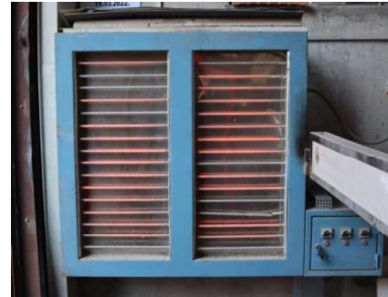
Fig. 4. Testing of surface spread of flame (SRPS U.J1.060)
