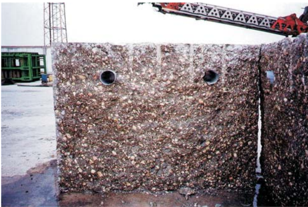
Figure 2 Cross-section of armour cube Slika 2. Poprečni presjek kocke
