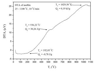
Figure 2: DTA curve of mullite Slika 2: DTA-krivulja mulita
