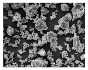
Figure 3: Mullite particles (SEM) Slika 3: SEM-posnetek zrn mulita
