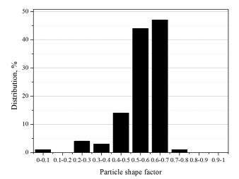
Figure 5: Distribution of the particle-shape factor of mullite Slika 5: Razporeditev faktorja oblike zrn mulita
