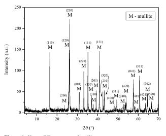
**Figure 1:** X-ray diffractogram of mullite **Slika 1:** Rentgenski difraktogram mulita
