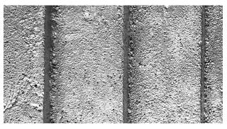
Figure 6: Appearance of the mullite-based lining on a test sample without visible flaws
