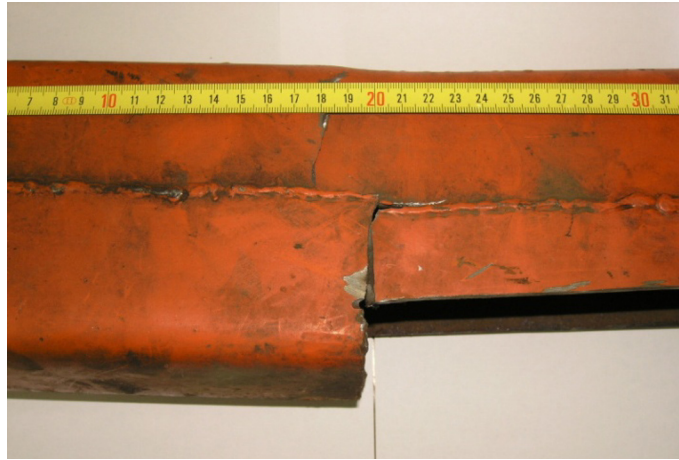
Fig. 7. Part of the damaged lever 3 used for sampling.
