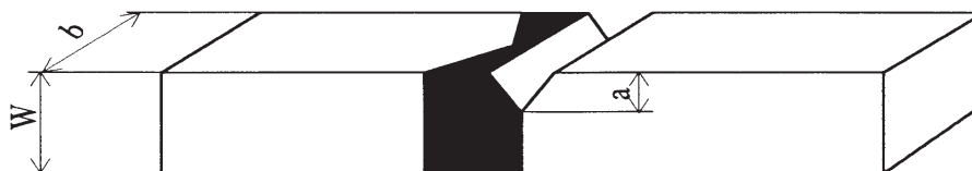
Figure 3: Dimensions of specimen and notch position.
