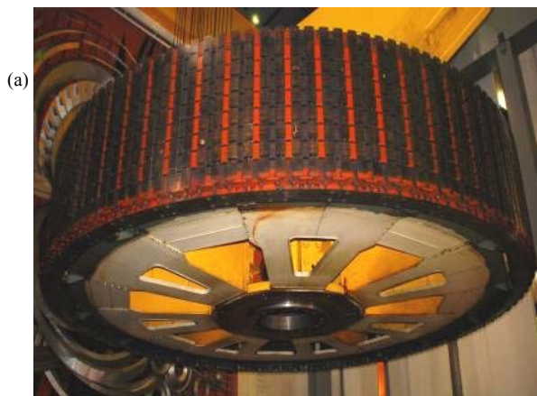
Figure 2. Parts of generator rotor hub station: a) rotor; b) hub; c) arms.
