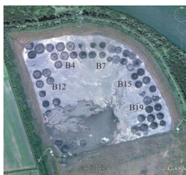
Fig. 1. Positions of the boreholes on the TENT-A landfill (source of the image Google Maps).
