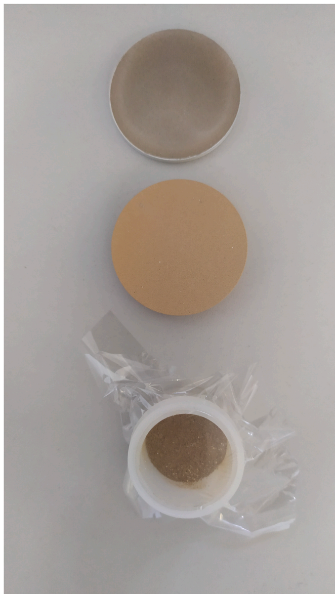
Fig. 1. Three approaches to the preparation of the samples: a) Loose powder preparation (LP), b) Pressed pellet preparation with binder wax (PPB), and c) Fired pressed pellet preparation without binder wax (FPP).
