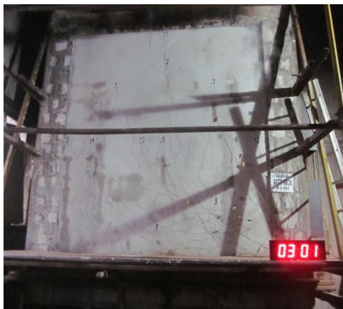
Figure 12. Unexposed fire side of a wall at the end of test
