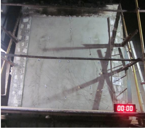
Figure 10. Unexposed fire side of a wall at the start of test
