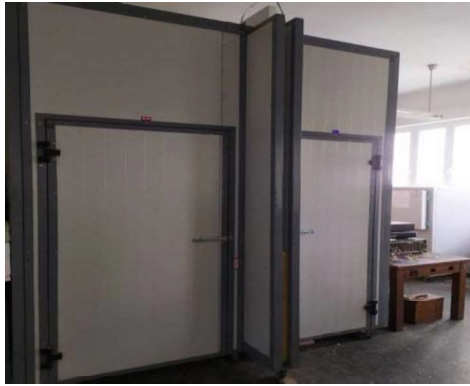
Figure 1: Test chamber according to SRPS U.J5.060
