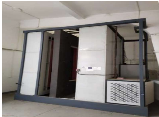
Figure 2: Test chamber according to SRPS EN ISO 12567-1
