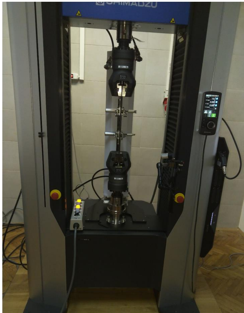
Figure 8. Tensile testing of wire sample.
