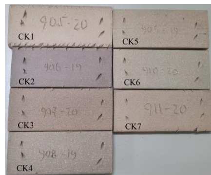
Figure 7. Macro appearance of samples fired at 1250 °C.
