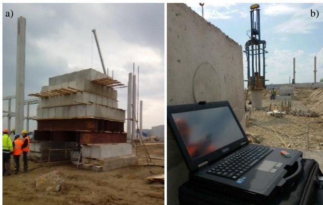
Figure 4. Pile no.2: a) SLT of pile; b) DLT of pile; c) force signals obtained by DLT.
