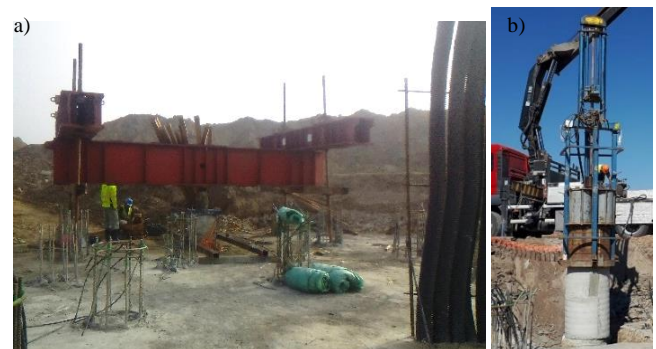
Figure 4. Pile no.2: a) SLT of pile; b) DLT of pile; c) force signals obtained by DLT.
