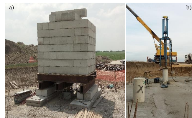
Figure 3. Pile no.1: a) SLT of pile; b) DLT of pile; c) force signals obtained by DLT.
