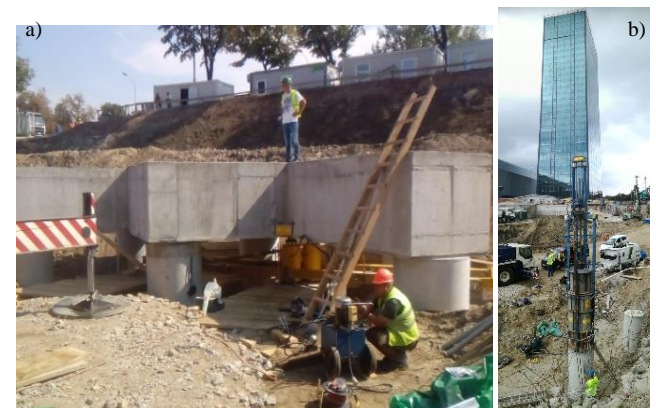
Figure 5. Pile no.3: a) SLT of pile; b) DLT of pile; c) force signals obtained by DLT.
