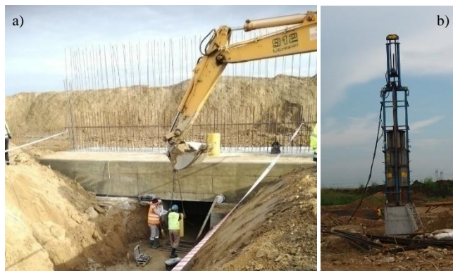
Figure 6. Pile no.4: a) SLT of pile; b) DLT of pile; c) force signals obtained by DLT.
