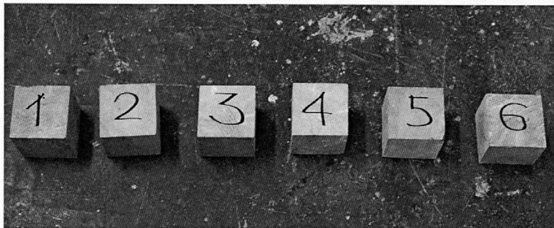
Figure 2. Samples prepared according to SRPS EN 1926 for compressive strength test
