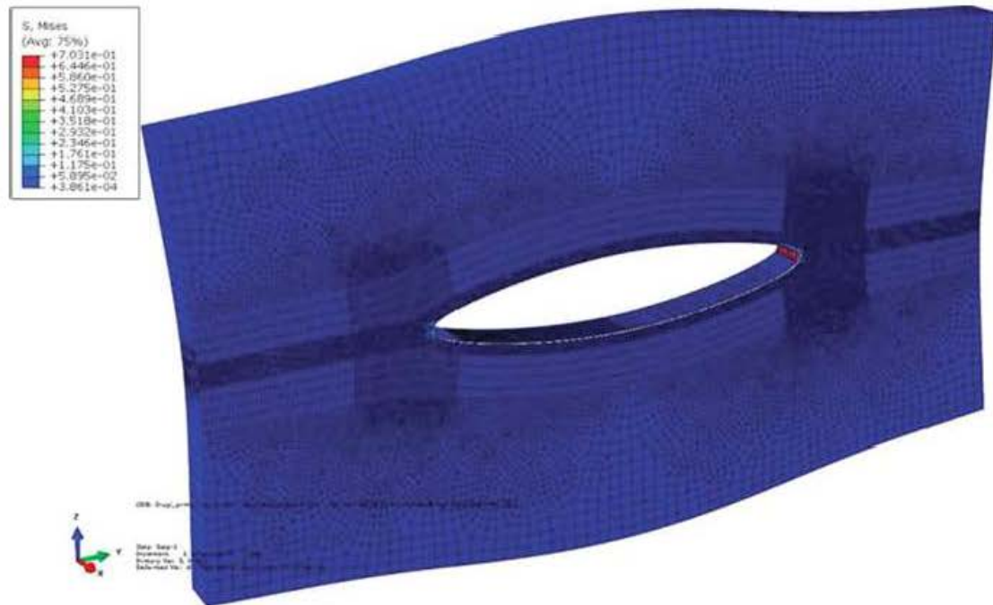
Fig. 5 Stress state (von Mises) of the plate after crack opening displacement (hexahedral elements)
