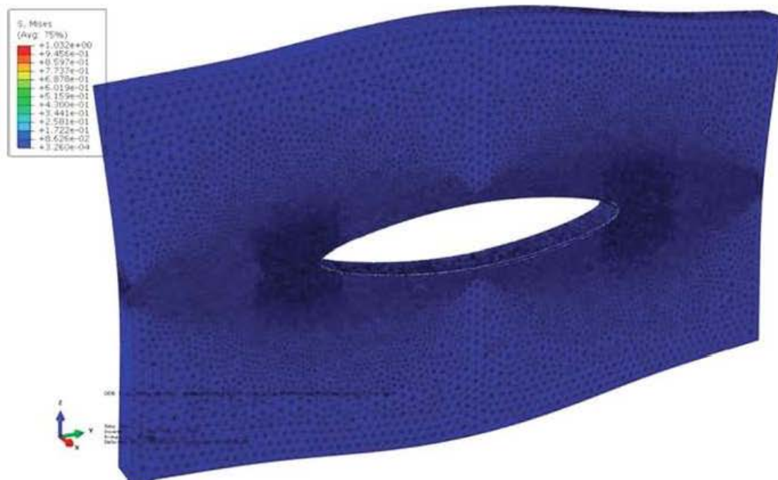
Fig. 7 Stress state (von Mises) of the plate after crack opening displacement (tetrahedral elements)
