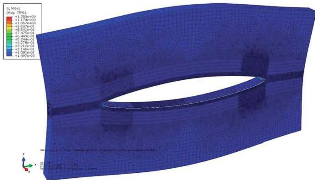
Fig. 9 Stress state (von Mises) of a plate after 18 steps of crack propagation (hexahedral elements)
