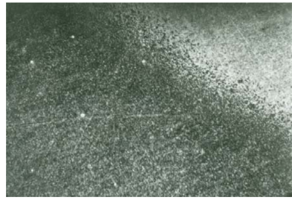
Figure 6. Transition zone, hardness values between 300 and 600 HV.
