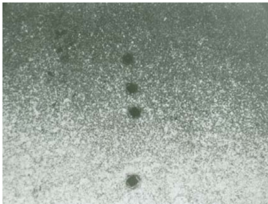
Figure 7. Fine grain ferrite-pearlite microstructure of chain bracket forging, average hardness value 220 HV.
