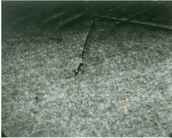
Figure 5. Carburized zone with the crack, hardness values between 600 and 700 HV.
