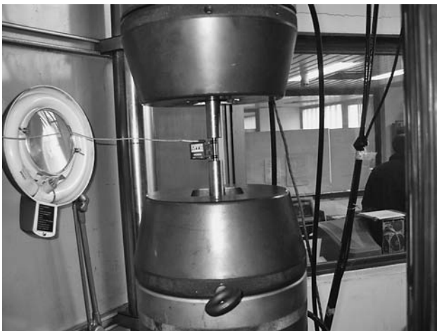
Figure 1 MTS extensometer during fatigue loading
