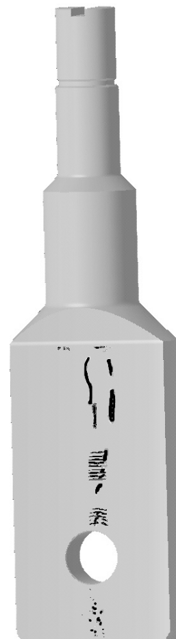
Figure 4. Indications of ultrasonic testing performed on the threaded spindle of the beam (upper view).
