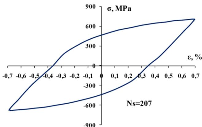
Figure 4. Example of stabilized hysteresis loop.
