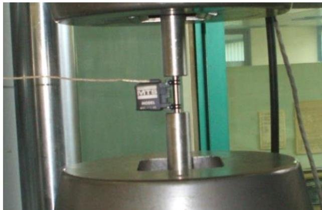
Figure 3. MTS extensometer.
