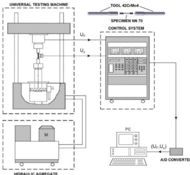
Figure 2. Overall scheme of the MTS testing system, /3/.
