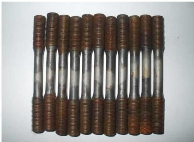
Figure 1. Round specimens prepared for LCF testing.
