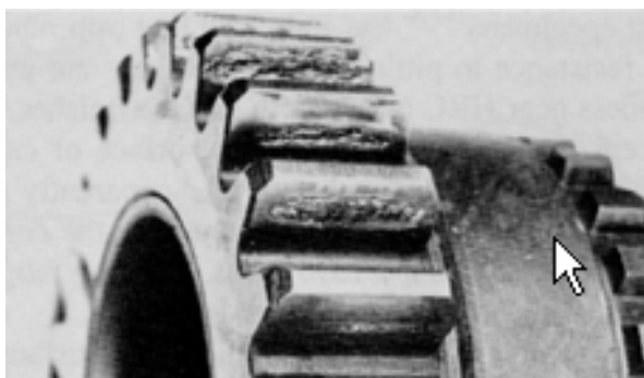
Slika 5. Piting boka zupca – početni (gore) i progresivni (dole) Figure 5. Tooth flank pitting – initial (up) and progressive (down)
