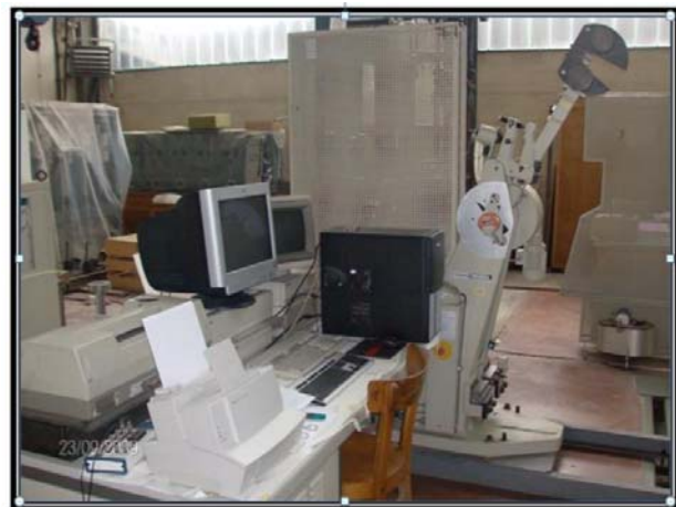
Fig. 2. SCHENCK TREBEL for impact testing
