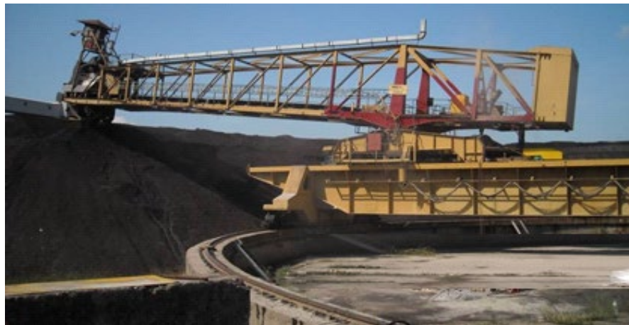
Figure 1. Bucket-wheel excavator DU1 at the coal landfill of the thermal power plant 'Nikola Tesla A'
