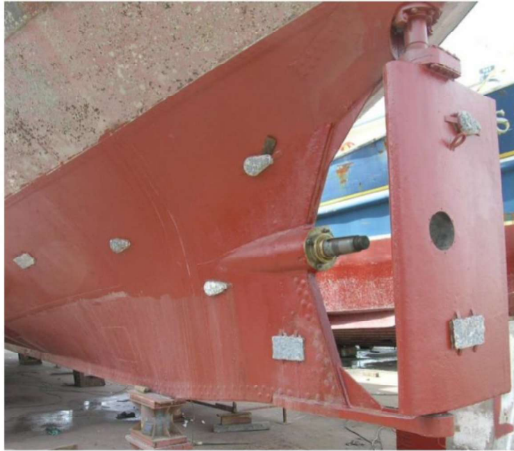
Figure 6. Cathodic protection using sacrificial anodes (zinc)
