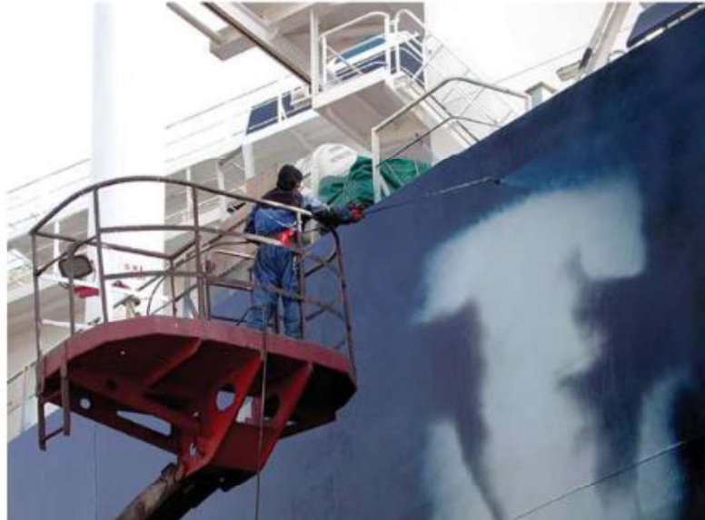
Figure 5. Airless spray application of paint onto the vessel's topsides
