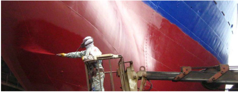
Figure 3. Corrosion protection with coatings
