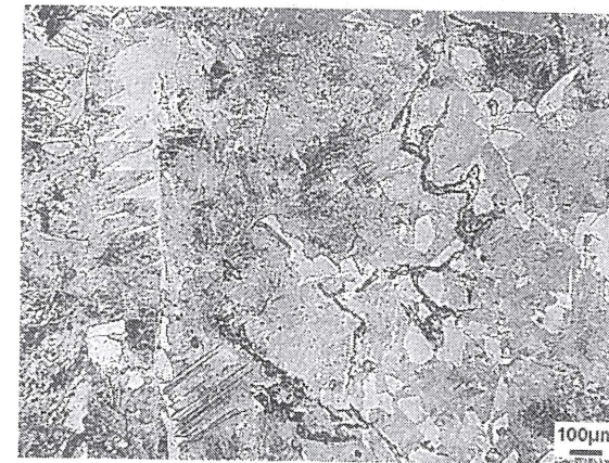
Fig. 3.8. Micro- and macro-cracks formed due to segregation in the material connecting rod. 4% natal.
